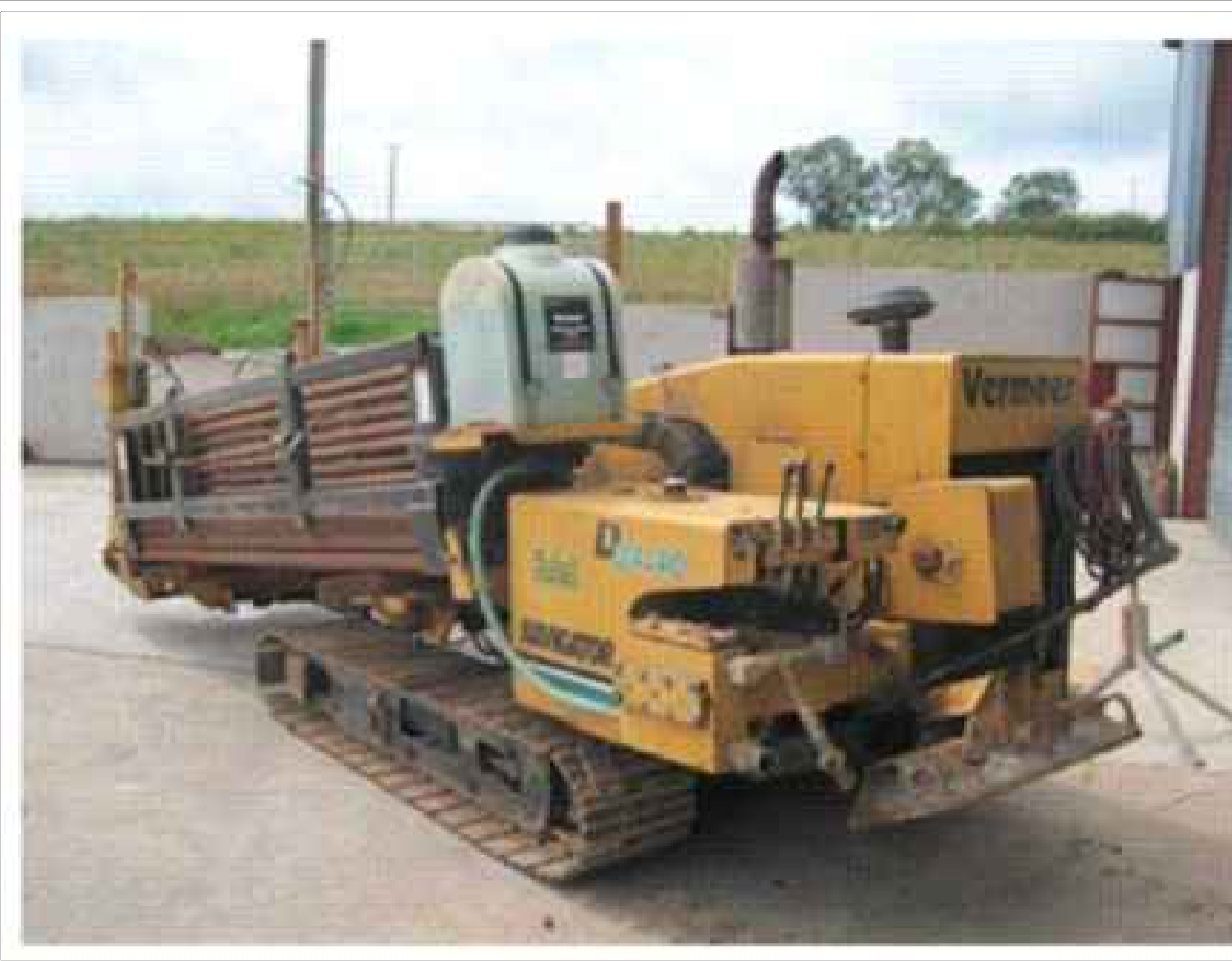
Image 2 | Typical Directional Drilling Rig
